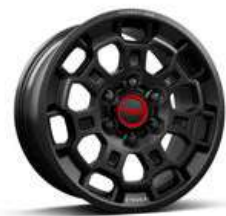
TRD Pro: 18-in. black forged-aluminum BBS ®14 wheels with TRD center caps
